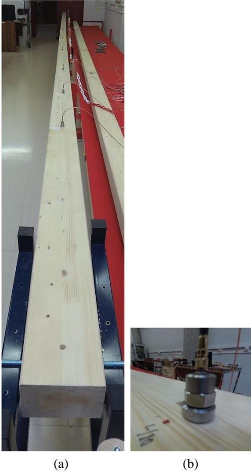
**Figure 1:** (a) Picture of the timber beam; (b) detail of an accelerometer
