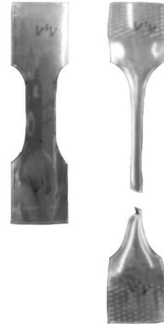
**Figure 1:** PET sample : before (left) and after (right) tensile strength test.
