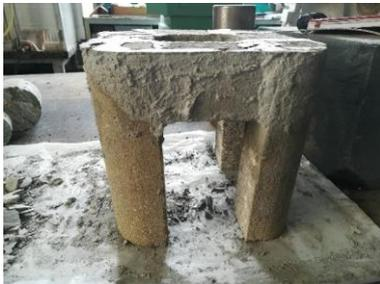
**Figure 1.** 3D frame bonded with mortar.
