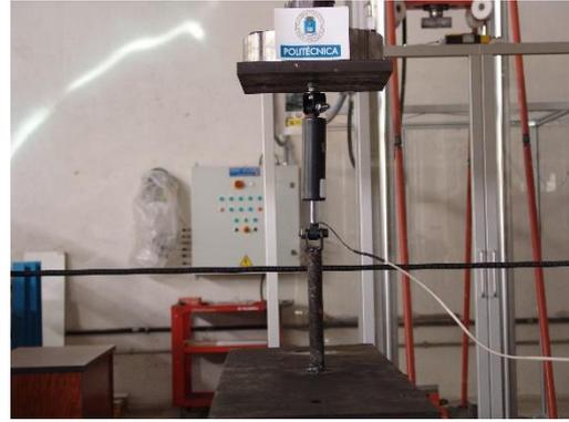
**Figure 4** : View of the MR Damper, joining to the concrete block and the hydraulic jack.
