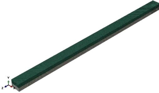
**Figure 1:** Steel-Concrete cantilever beam. Concrete green color. Steel grey color.
