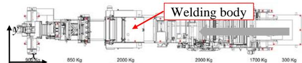
Figure 3: Plan view of the vibrating machine
