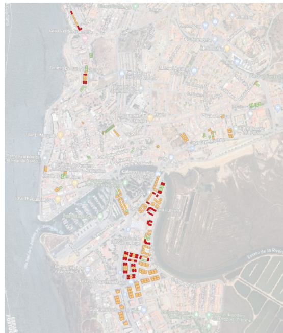
Figure 7: Expected damage state for a seismic event of intensity VII. Slight (green), Moderated (orange) and Heavy (red).
