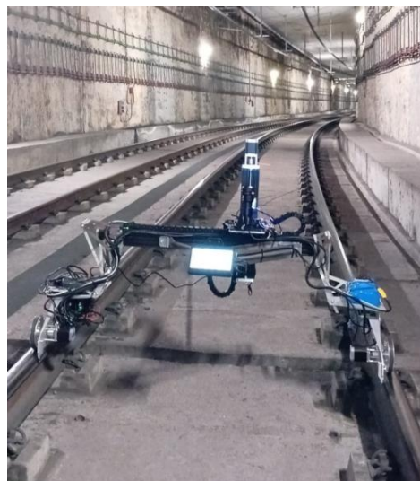
Figure 3. Measuring device positioned on the rails of the Malaga Metro track.
