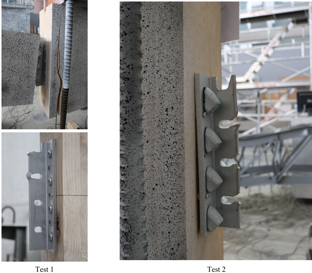
Figure 9: Mode of failure identified for each Test.
